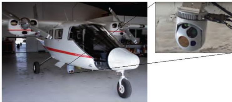
Figure 4. P68 Observer aircraft outfitted with multi-spectral camera.
